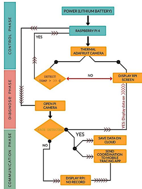
Fig. 12. Flow Chart System Architecture.
