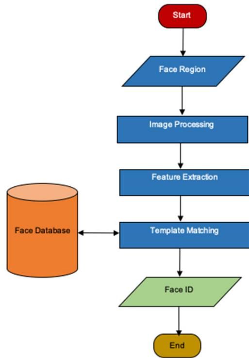
Fig. 14. Face recognition algorithm flow chart.
