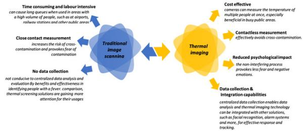
Fig. 3. Features comparison of the traditional image scanning and thermal imaging [15].
